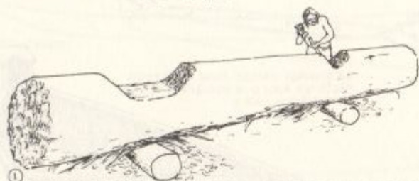
① CANOEMAKER REMOVED BARK FROM CEDAR LOG AND CHISELLED OUT SECTION FROM EACH END.
