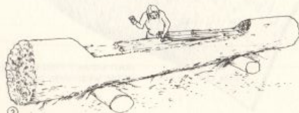
② HE SPLIT OUT WOOD FROM BETWEEN CUTS, USING WEDGES AND HAND MAUL.
