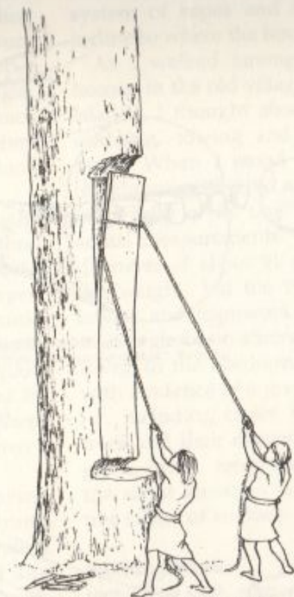
PULLING ON ROPE HELPED TO SPLIT PLANK AWAY FROM TRUNK. WC X PERS.COMM, RON HAMILTON.
